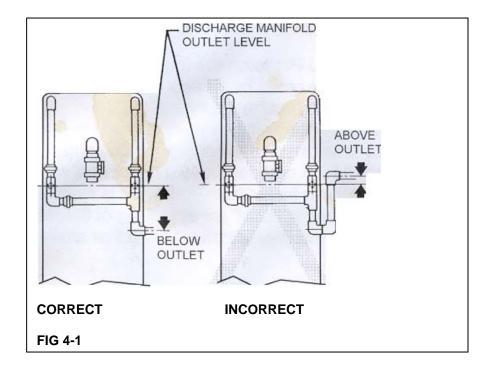
**CAUTION:** The filtrate drains from the press by gravity. Therefore the outlet of the drain pipe must be below the level of the discharge manifold outlet.
