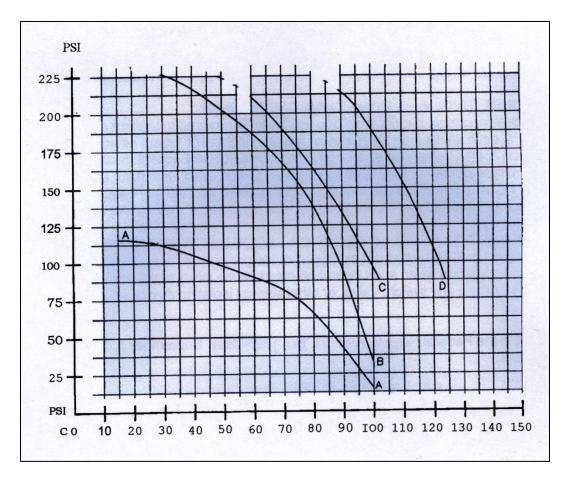
"A" = Low Pressure Plates, Standard 100 psi design, Polypropylene "B" = High Pressure Plates, Polypropylene
