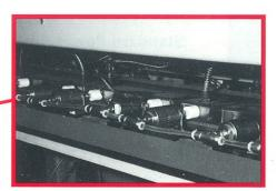
Five separate heater bars follow bag contour for maximum heat transfer and optimum seal.
