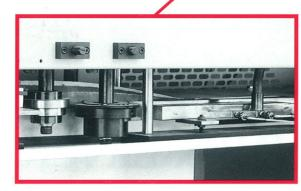
The unique heater manifold system reactivates pre-applied adhesive uniformly to ensure a proper seal.
