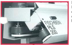
Fischbein's patented Breakaway design eliminates costly downtime caused by bag jamming.
